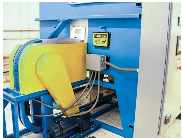
Fig. 5. Quick load-transfer system (courtesy of Wisconsin Oven Corp.)
