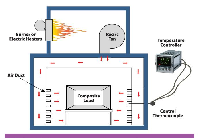
The flow of recirculated air, shown with red arrows, is demonstrated in this section view of a composite cure oven.
