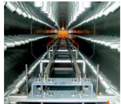
▲ Sand core dryers use high-velocity air nozzles to improve energy efficiency by allowing a reduced oven temperature.
