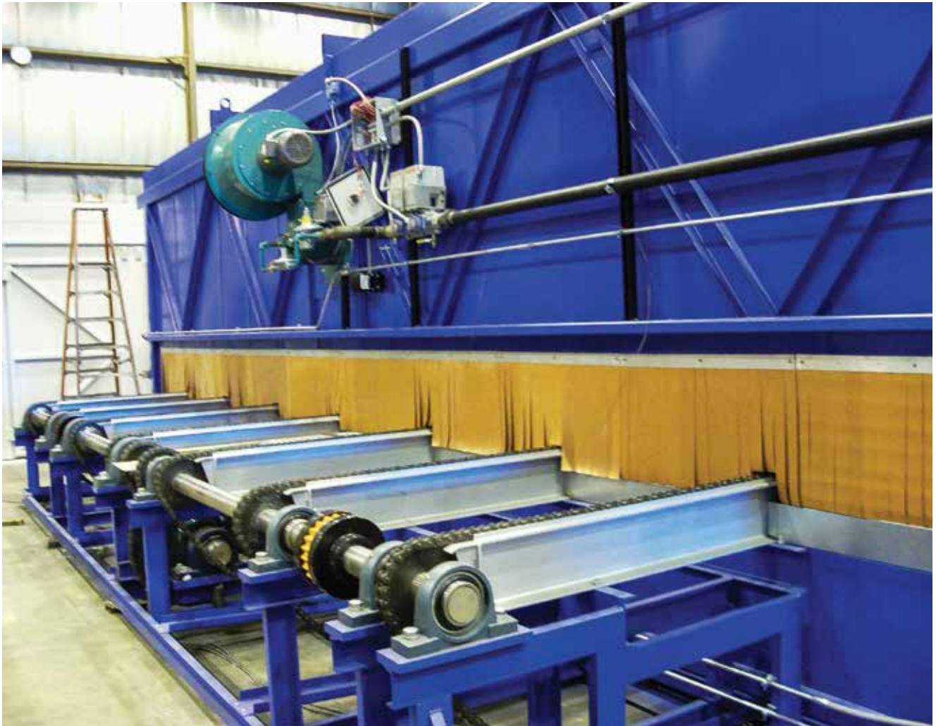
FIGURE 4. Some wood-drying ovens use a multiple-strand chain conveyor system.
